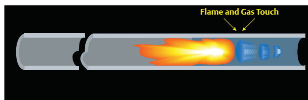
Figure 14. Concept of deflagration-to-detonation transformation in a pipe.
